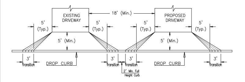
IF DISTANCE BETWEEN TWO ADJACENT DRIVEWAYS IS LESS THAN 18', REDUCE THE 5' FLARES TO ALLOW FOR A MINIMUM OF 2' OF FULL HEIGHT CURB BETWEEN TRANSITIONS. IF DISTANCE BETWEEN DRIVEWAYS IS LESS THAN 8', THE TRANSITIONS AND 2' OF FULL HEIGHT CURB WILL NOT FIT. IN THIS INSTANCE, SPECIAL DETAILS MAY BE REQUIRED. IN INSTANCES WHERE THE DISTANCE SEPARATING DRIVEWAYS IS BETWEEN 8' AND 18', USE THE DETAIL BELOW:
